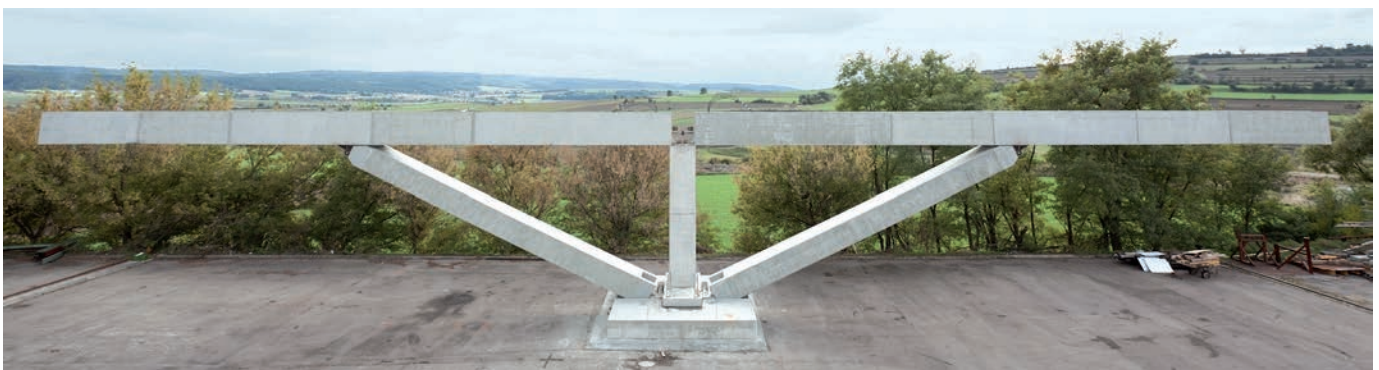
Fig. 17. Large-scale model of the balanced lift part of the Lafnitz Bridge
